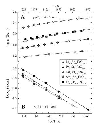
**Figure 7.** Temperature dependencies of the total conductivity of  $\text{Ln}_{0.5}\text{A}_{0.5}\text{FeO}_{3-\delta}$  at atmospheric oxygen pressure (A) and n-type electronic conductivity at  $p(O_2)=10^{-15}$  atm (B).
