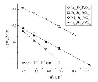
**Figure 12.** Temperature dependence of the oxygen-ionic conductivity of  $Ln_{0.5}A_{0.5}FeO_{3-\delta}$  calculated from the  $p(O_2)$  dependencies of the total conductivity under reducing conditions.
