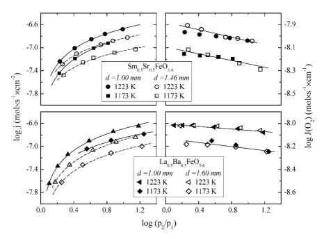
Figure 9. Dependence of the oxygen permeation fluxes (left) and specific oxygen permeability (right) of  $Sm_{0.5}Sr_{0.5}FeO_{3-\delta}$  and  $La_{0.5}Ba_{0.5}FeO_{3-\delta}$  ceramic membranes on the oxygen partial pressure gradient. The feed-side oxygen pressure ( $p_2$ ) is 0.21 atm.
