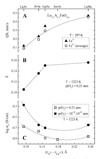
**Figure 5.** Room-temperature quadrupole splittings of Fe<sup>3+</sup> and Fe<sup>4+</sup> signals (A), oxygen nonstoichiometry at 1223 K and atmospheric oxygen pressure (B), and ionic conductivity values at 1223 K in air and in reducing atmospheres (C) vs the difference between A<sup>2+</sup> and Ln<sup>3+</sup> cation radii. The radius values<sup>34</sup> correspond to 9-fold coordination. All lines are a guide for the eye.
