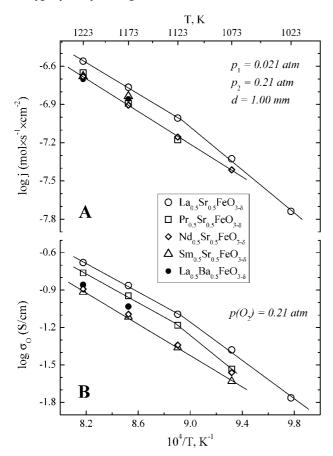
Figure 11. Temperature dependencies of the oxygen permeation fluxes through Ln<sub>0.5</sub>A<sub>0.5</sub>FeO<sub>3-δ</sub> membranes under fixed oxygen partial pressure gradient (A) and oxygen ionic conductivity at atmospheric oxygen pressure (B). Solid lines are for visual guidance only.
