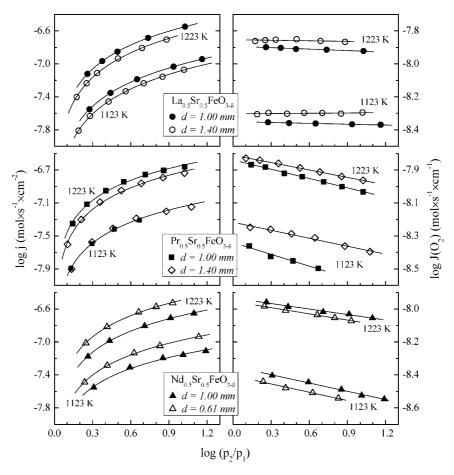
Figure 8. Dependence of the oxygen permeation fluxes (left) and specific oxygen permeability (right) of dense  $Ln_{0.5}Sr_{0.5}FeO_{3-\delta}$  (Ln = La-Nd) ceramic membranes on the oxygen partial pressure gradient. The feed-side oxygen pressure ( $p_2$ ) is 0.21 atm.
