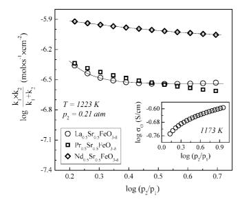
**Figure 10.** Example of the surface exchange coefficients of  $Ln_{0.5}Sr_{0.5}FeO_{3-\delta}$ (Ln = La-Nd), estimated by eq 2 from the oxygen permeation data. Inset shows the calculated ionic conductivity of La<sub>0.5</sub>Sr<sub>0.5</sub>FeO<sub>3- $\delta$ </sub>, averaged under the oxygen partial pressure gradient, at 1173 K.
